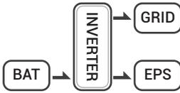
On discharge time, if load power is less than battery power, battery will supply power to loads as first priority, the excess power will be fed to grid.
