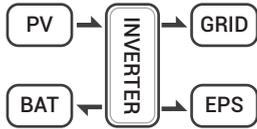
On charge time, solar energy will charge battery as first priority. The excess energy will supply power to the loads. If solar energy is sufficient to supply loads and charge battery, and if there's still some extra energy, then the excess power will feed the power to grid.
