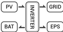
Solar energy will charge battery as first priority, if solar energy is excess.
