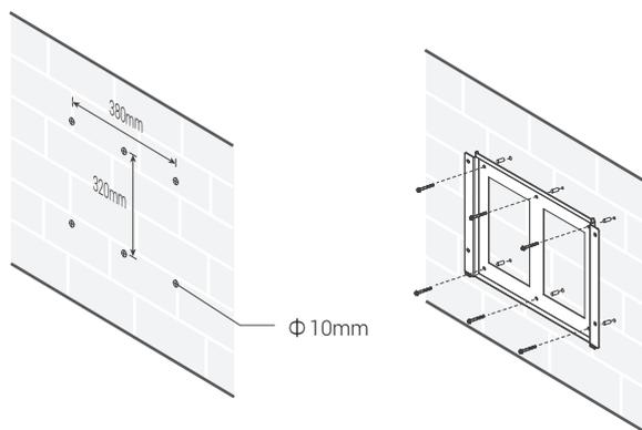
**Step 2:** Use the screws to fix the crossbar as shown in the figure below.
