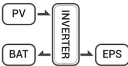
Solar energy provides power to the loads as first priority .if solar energy is sufficient to power all connected loads, solar energy will provides to charge battery.
