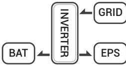
On charge time, grid will charge battery and supply power to the connected loads at the same time.
