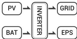
On discharge time, solar energy provides power to the loads as first priority, if solar energy is sufficient to supply loads, and if there's still some extra energy from solar energy, then the excess power and battery will deliver the power to the grid at the same time.
