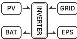
Solar energy will charge battery as first priority, if solar energy is excess the excess power will supply load.
