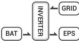
On discharge time, if load power is more than battery power, battery and grid will supply power to the loads at the same time.
