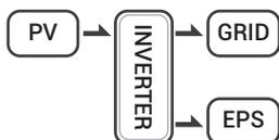
In the period of no charge or discharge, the solar power supply loads at first priority, excess energy to the grid.
