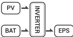
Solar energy provides power to the loads as first priority.if solar energy is not sufficient to power all connected loads, battery energy and solar energy will supply power to the loads at
