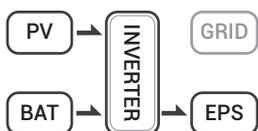
Solar energy provides power to the loads as first priority, if solar energy is not sufficient to power all connected loads, battery energy will supply power to the loads at the same time.
