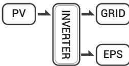
Solar energy provides power to the loads as first priority.if solar energy is Inverter sufficient,the excess power will feed to grid.
