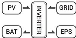
On charge time, solar energy will charge battery as first priority, then the excess solar energy will supply power to loads. If solar energy is not sufficient to charge battery and supply loads, grid will supply all the connected loads with solar energy together.
