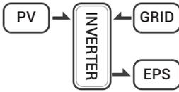
Solar energy provides power to the loads as first priority, if solar energy is not sufficient to power all connected loads, Grid energy will supply power to the loads at the same time.
