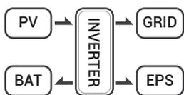
Solar energy provides power to the loads as first priority. If the solar energy is sufficient to power all connected loads, then the surplus solar energy will charge the battery. The remaining energy will be fed into the grid.
