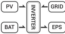
Solar energy provides power to the loads as first priority, if solar energy and battery are not sufficient to power all connected loads, utility energy (Main Grid) will supply power to the loads with solar energy at the same time.
