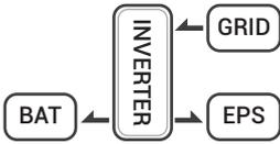
Grid will supply power to load and charge battery at the same time.
